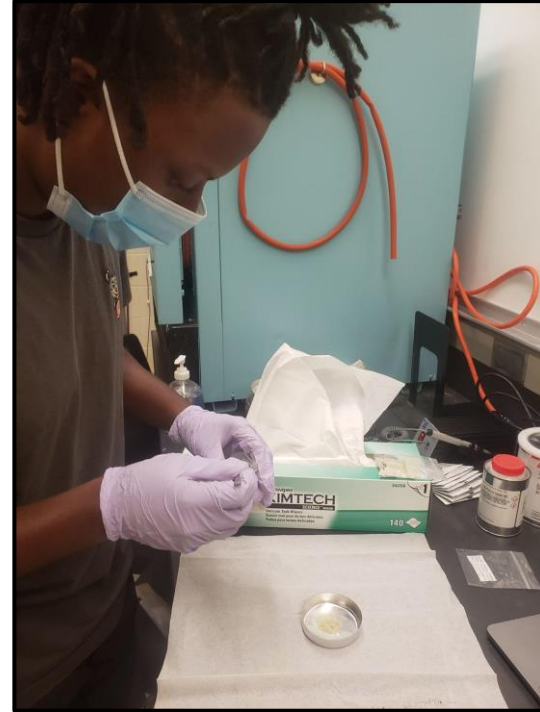
Me Mixing the Resin with the 2.4 and 20 um Diamonds
