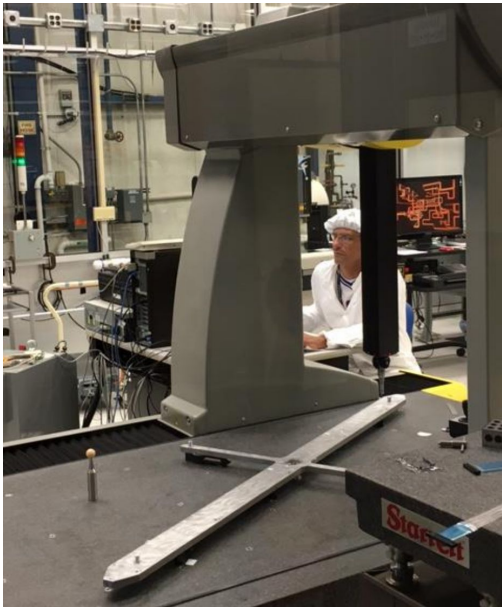
CMM of DSFM propeller (kinematic mounting features, ...)
