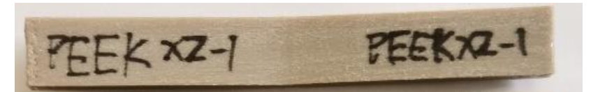
Sample built in XZ-direction after test
