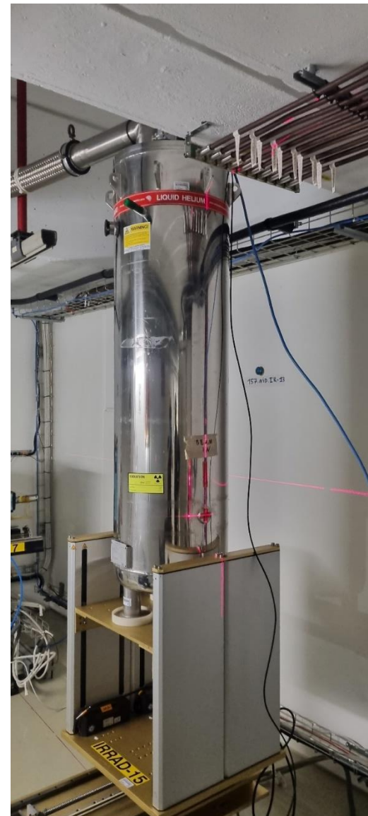
Cryostat for proton irradiation in liquid helium
