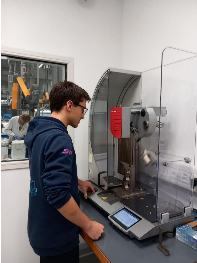
Zwick HIT5.5P impact tester for Dynstat tests
