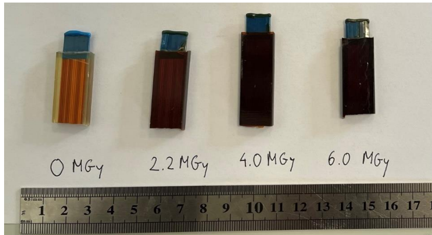
Ribbon cables impregnated with Araldite G 285 + Jeffamine D400 before and after irradiation up to 6 MGy.
