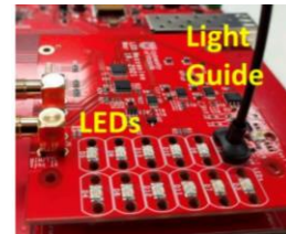
LED Light Sources Inside the multi-PMT Module
