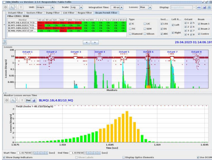
Loss structure due to beam-dust interaction on 29.04. causing the quench of a main dipole
