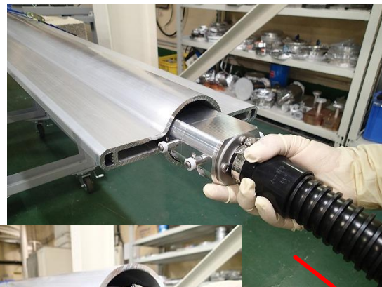
Special tool to cleanup the bottom of beam channel
