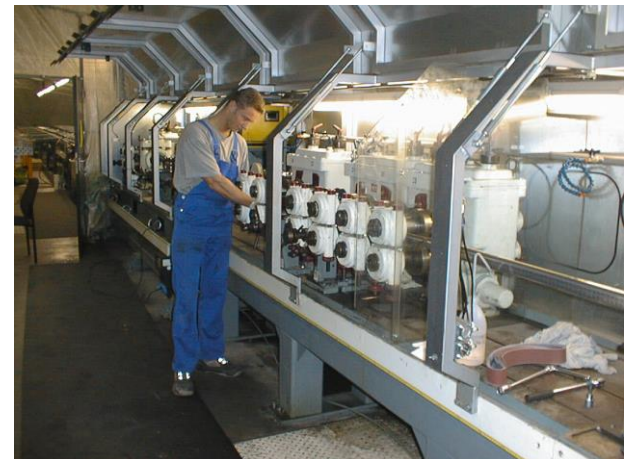
Beam screen tube production line
