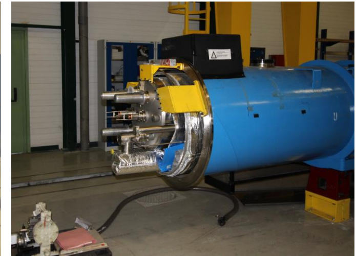
Beam screen insertion in a LHC dipole
