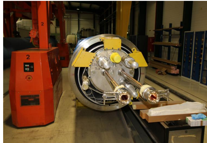
Beam screen insertion in a LHC dipole
