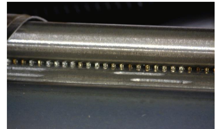
Spot laser weld of the cooling tube to the beam screen tube
