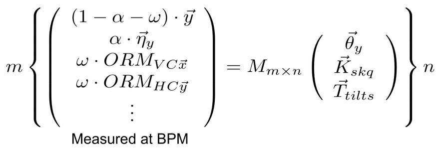
+ 2 (or more) columns of the off diagonal Orbit Response Matrix, being the vertical orbit generated by a Horizontal correctors (HC) and vice versa.
