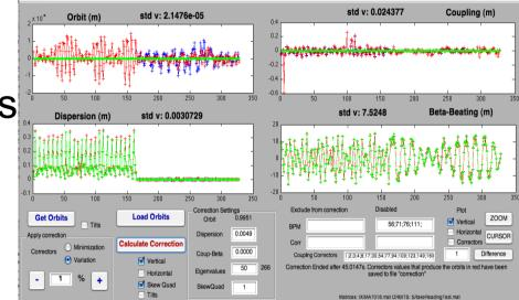
Monitor tilts (previously measured by LOCO) are taken into account in all measurements.
