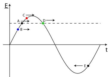
they arrive at the cavity. Here A is the synchronous particle, B is a one having higher energy, C is a particle with lower energy, D is a particle on the edge of phase stability and the particle E experiences a <u>retarding potential</u>.
