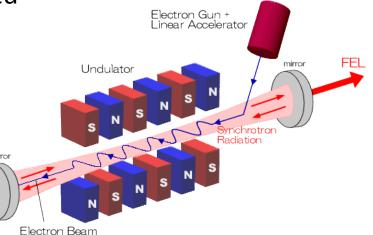
*radiates like one super-particle*. Radiated power with two components: *incoherent*  $P \sim Ne^2$  and *coherent*.  $P \sim N^2e^2$
