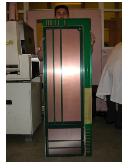
Early ATLAS NSW R&D Joerg Wotschack 1.5m x 0.5m plane Single panel
