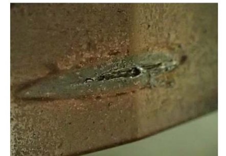
Damage to coated collimator jaw due to accidental beam loss in the SuperKEKB – T. Ishibashi ( talk )
