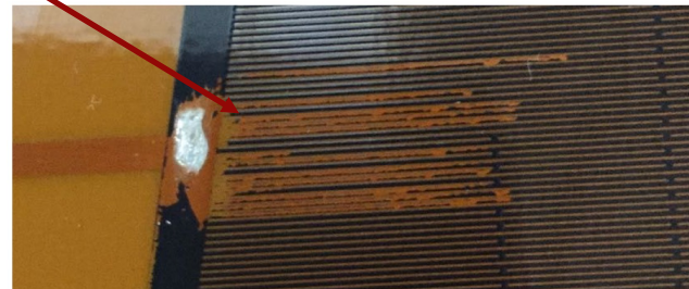
Foil with resistive pattern partially removed
