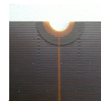
Central upper hole for layer interconnection. Readout strips routed around the hole. Central separation of resistive pattern.
