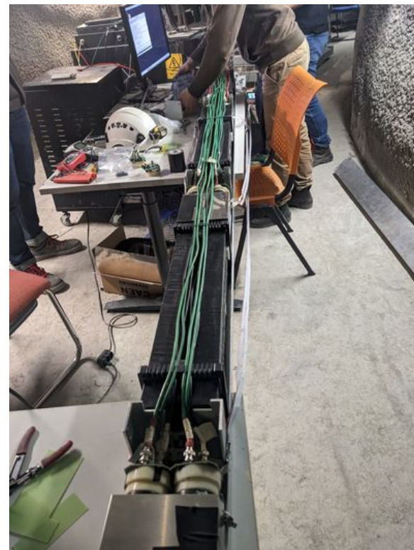
Supermodule assembly using 4 units
