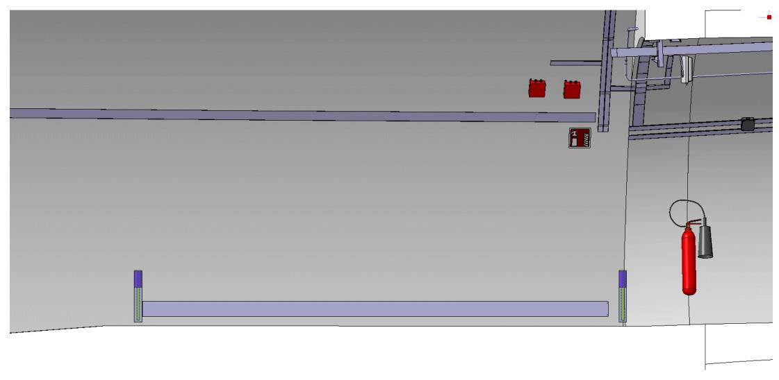
Transport space between installed detector and concrete shielding ~1.6m – sufficient.
