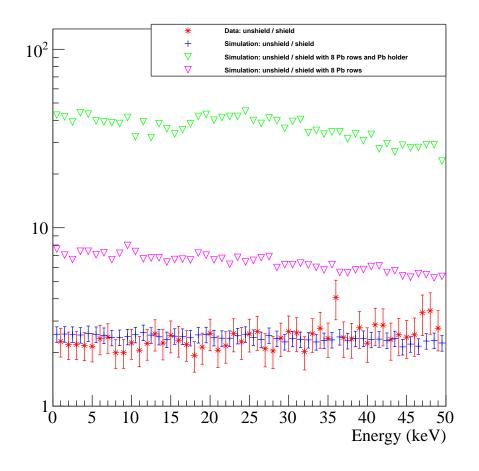
• Replacement of the waffer holder and 8 rows of Pb would reduce gamma contribution by nearly two orders of magnitude Monte Carlo simulations for the underground experiment at Gran Sasso
