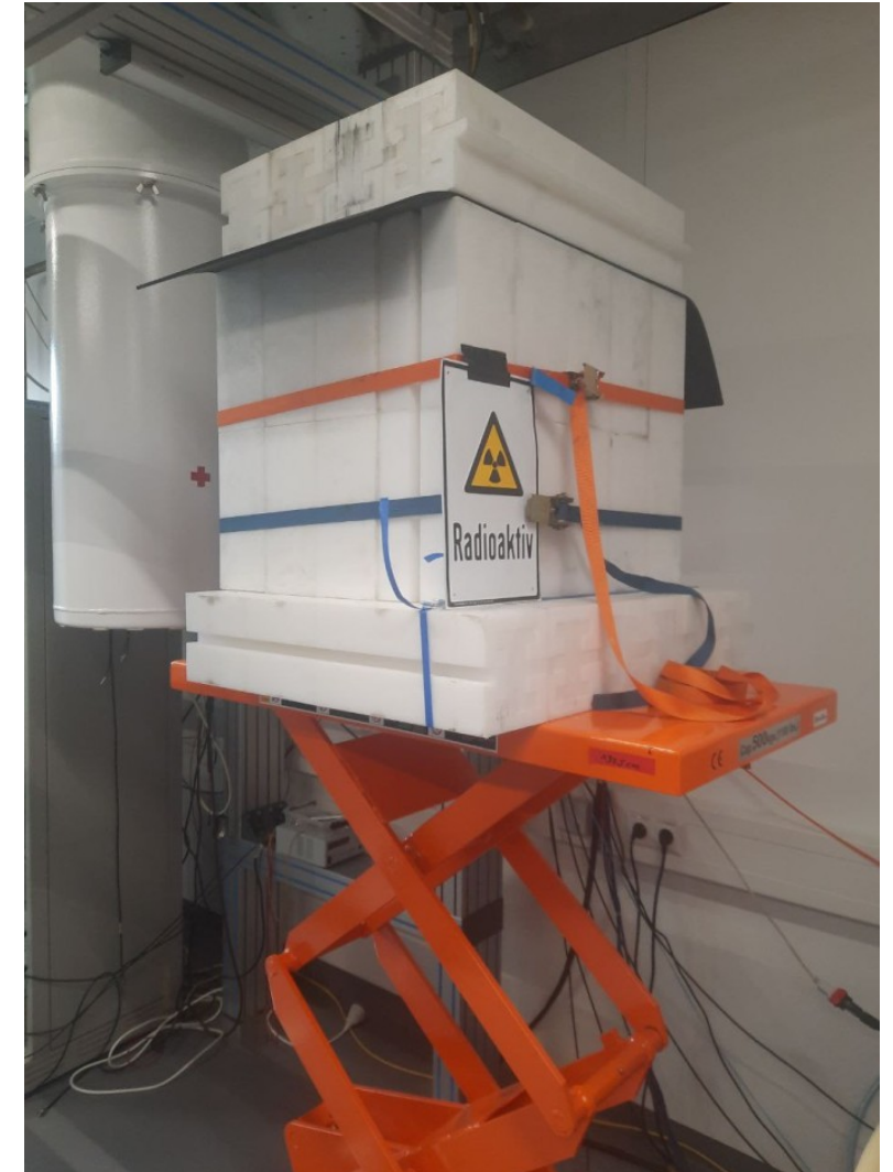
Thermal neutrons produced with a 3.7 MBq ^{252}\text{Cf} in a polyethylene and graphite moderator \Rightarrow 0.25 \text{ n}_{\text{th}}/\text{s} on the cryo-detector
