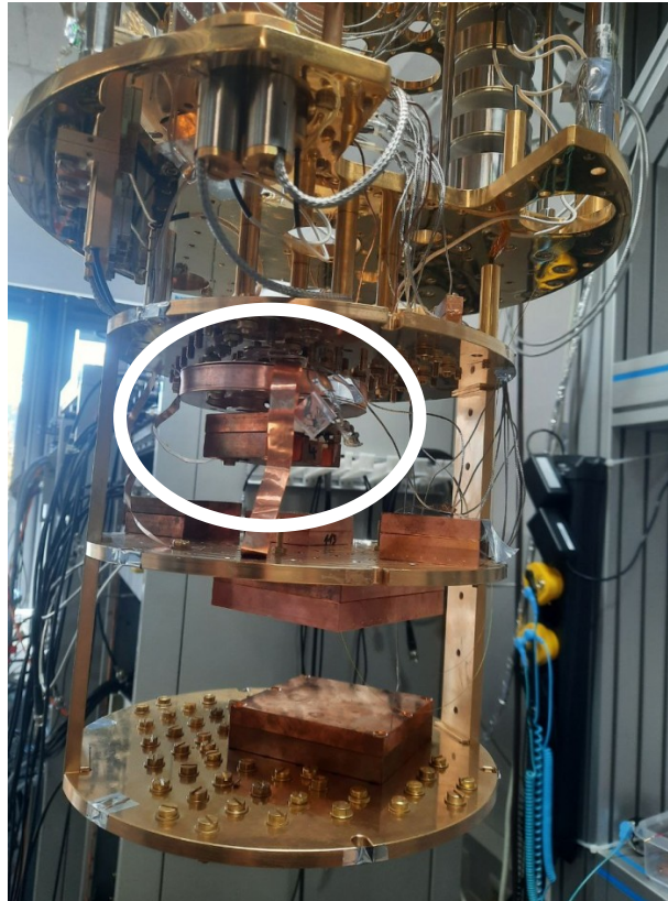
Detector in a copper box spring decoupled from cryostat vibration
