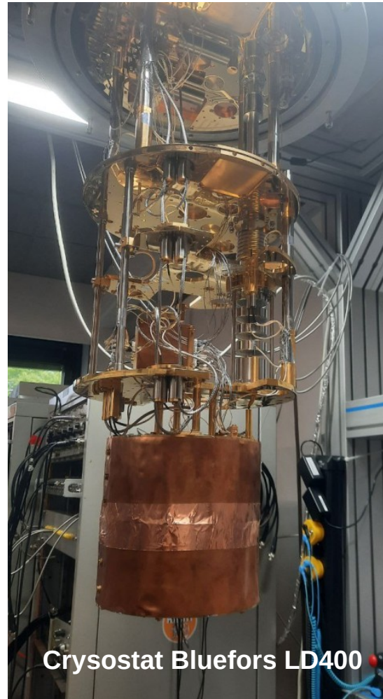
More copper to thermalize the detector below 100 mK TES transition ~10 mK
