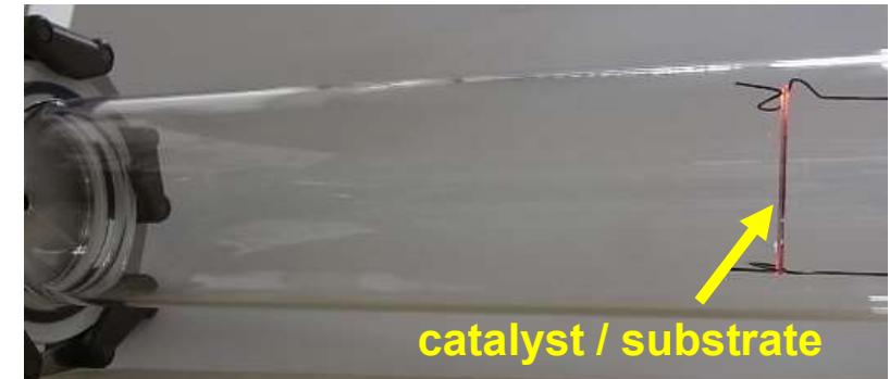
Gas-phase reaction & deposition on the reactor wall are suppressed.
