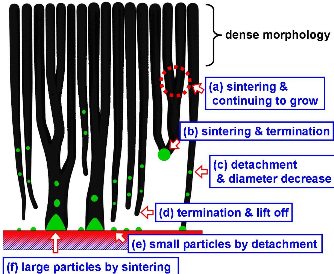
Several kinds of structural change of the catalyst nanoparticles occur simultaneously.
