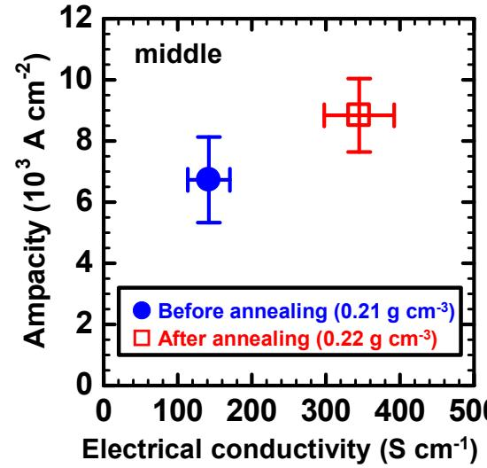
The electrical conductivity enhanced more significantly compared with the ampacity by annealing
