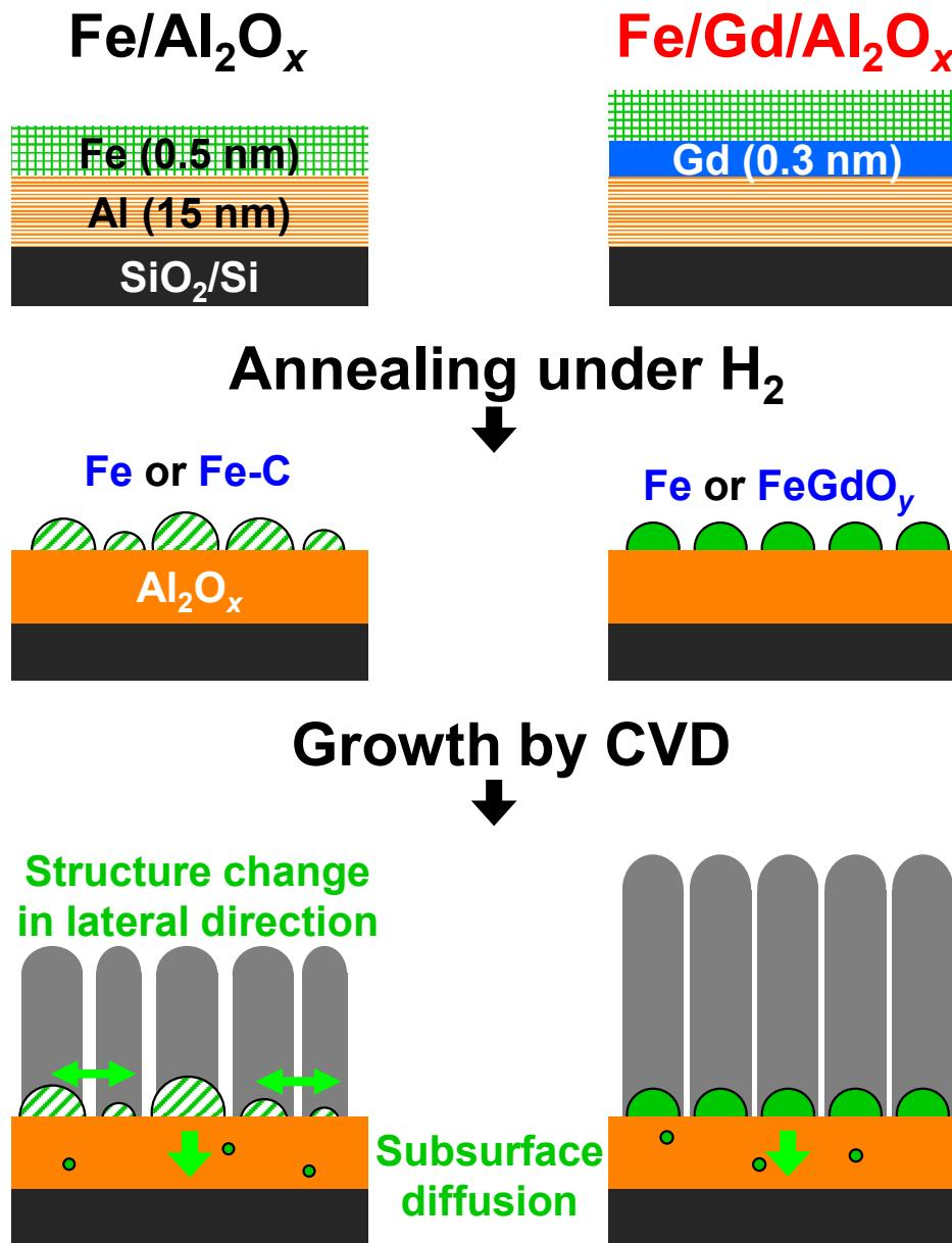
Structural change of the catalyst nanoparticles in lateral direction was suppressed by adding Gd.
