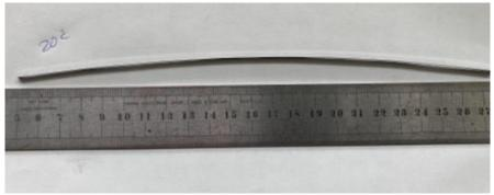
@20C radius is about 700mm silicon is on inner radius
