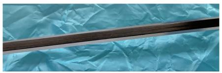
Glued 0.1x2mm carbon to 0.05x3mm silicon cured on 80C
