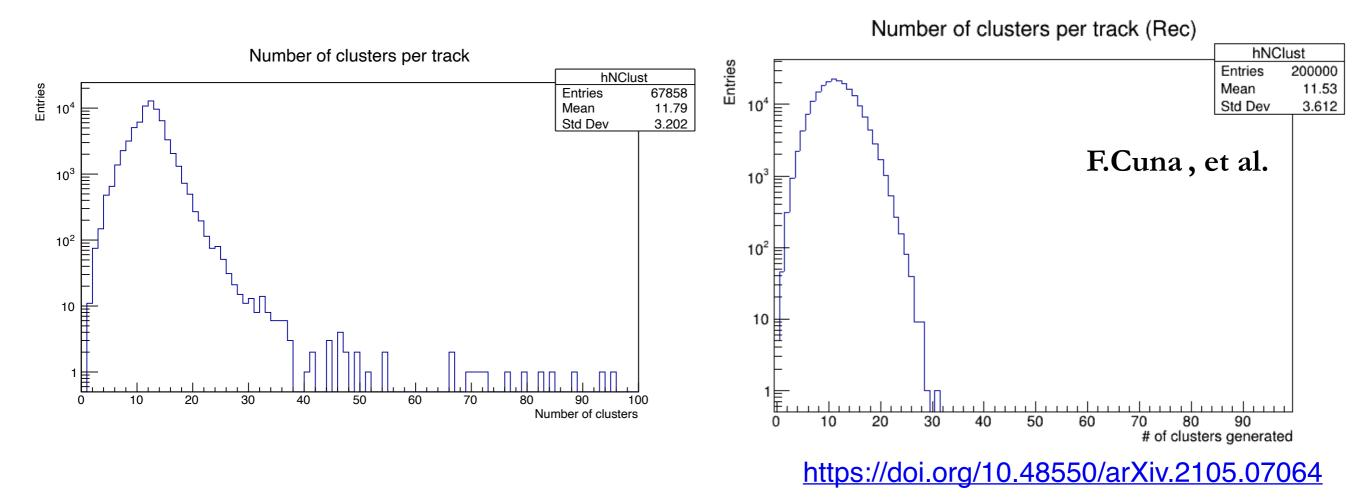
Gluster size distribution, for a muon at 300 MeV traversing 200 cells, 1 cm per side, filled with 10% He and 90 % iC₄H₁₀,
