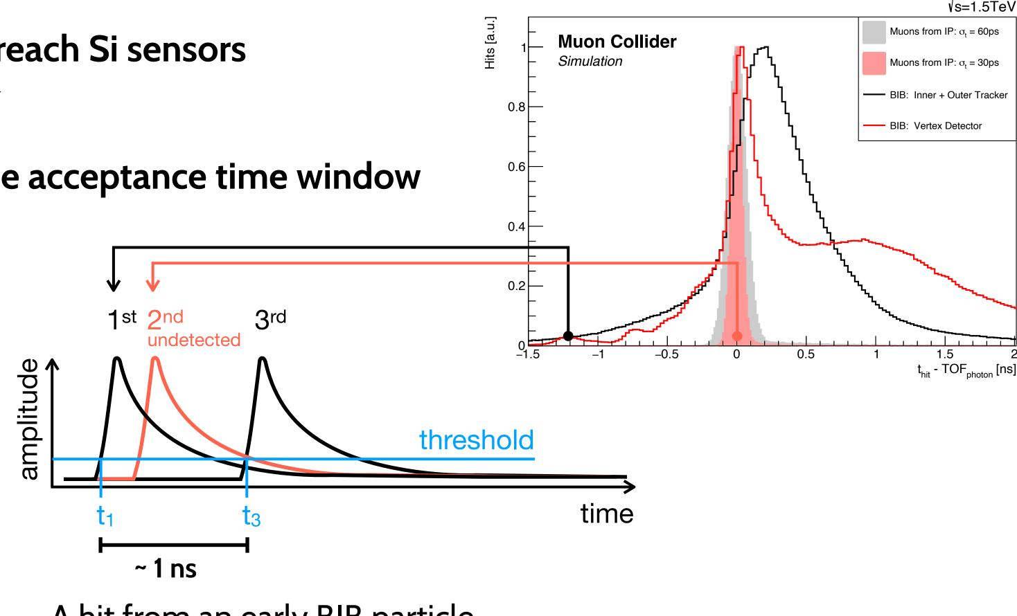
A hit from an early BIB particle makes the pixel "blind" to the potential signal particle arriving later
