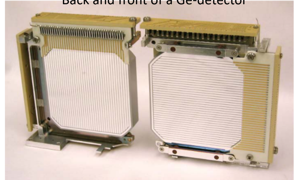
Back and front of a Ge-detector
