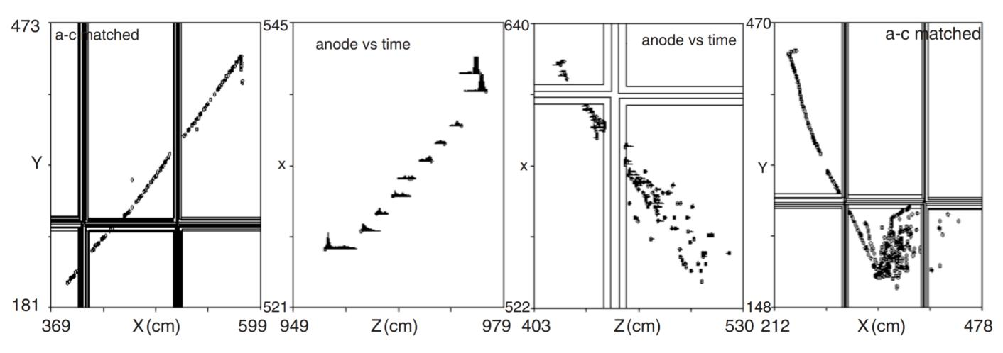
**Figure 9.** Example event displays from the Soudan-2 detector, showing the long track from a muon and a shorter, more heavily ionizing track from a recoil proton.
