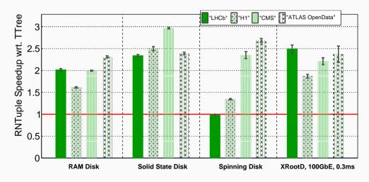
Single-core analysis throughput using RDataFrame
