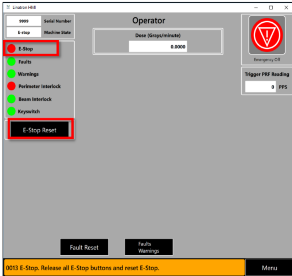
Figure: 3.9 Operator screen red E-stop indicator highlighted
