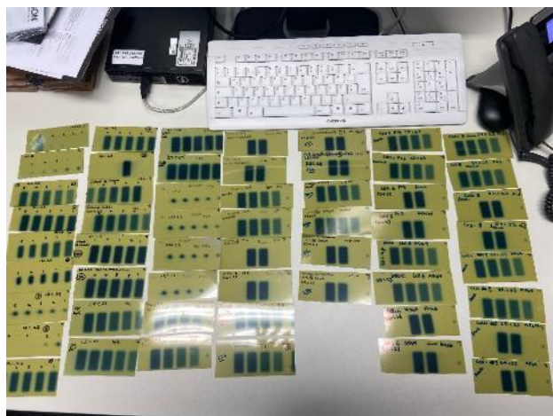
Dose calibration with dosimetry films and water phantoms
