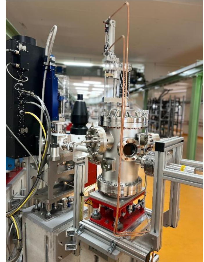
In low pressure vacuum, FH & M detector test stand.
