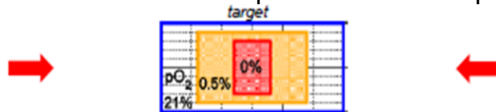
Example of the 'anoxic' phantom
