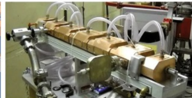
Fig. 4. TOP-IMPLART SCDTL structure: (left) schematic (right) 18-24 MeV booster built for the SPARKLE Company.
