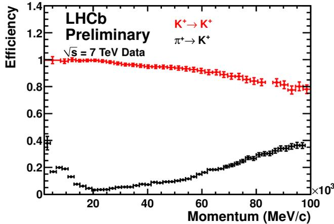
Figure 2: The RICH  $\pi/K$  separation performance as a function of momentum.
