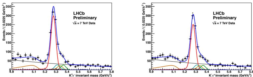
Figure 6:  $B^0 \rightarrow K\pi$  events selected in the 2010 LHCb data. Left  $K^+\pi^-$  and right  $K^-\pi^+$  selection. The fitted signal component is the dominant red curve. The difference in yields between  $K^+\pi^-$  and  $K^-\pi^+$  is driven by the direct CP-violation in the decay. The other curves show the contribution of background components. [20].
