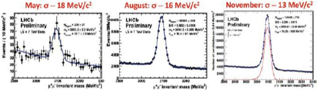
Figure 1: The  $\mu^+\mu^-$  invariant mass distribution in the  $J/\psi$  region.
