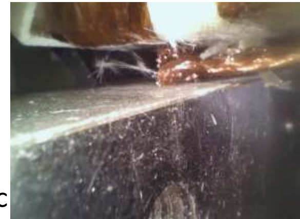
Finding the insulation fault with a grounded copper braid. Image credit Sandrine Le Naour 19
