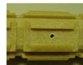
Fig. 5: One of the four sides of a sector at which a pick-up coil is fixed.
