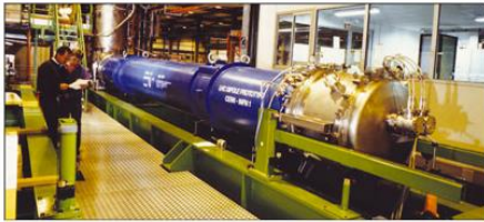
Fig. 7. On 14 April 1994 the first 10 m LHC dipole prototype from INFN was successfully powered at CERN for the first time. This magnet is now operating in the CAST experiment at CERN.
