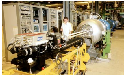
Fig. 7. On 14 April 1994 the first 10 m LHC dipole prototype from INFN was successfully powered at CERN for the first time. This magnet is now operating in the CAST experiment at CERN.
