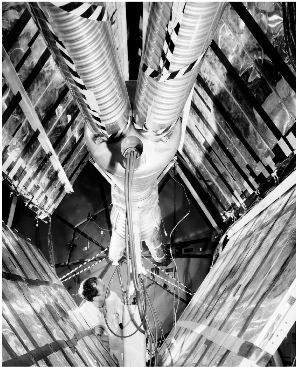
A vacuum chamber where the proton beams collide in the ISR
