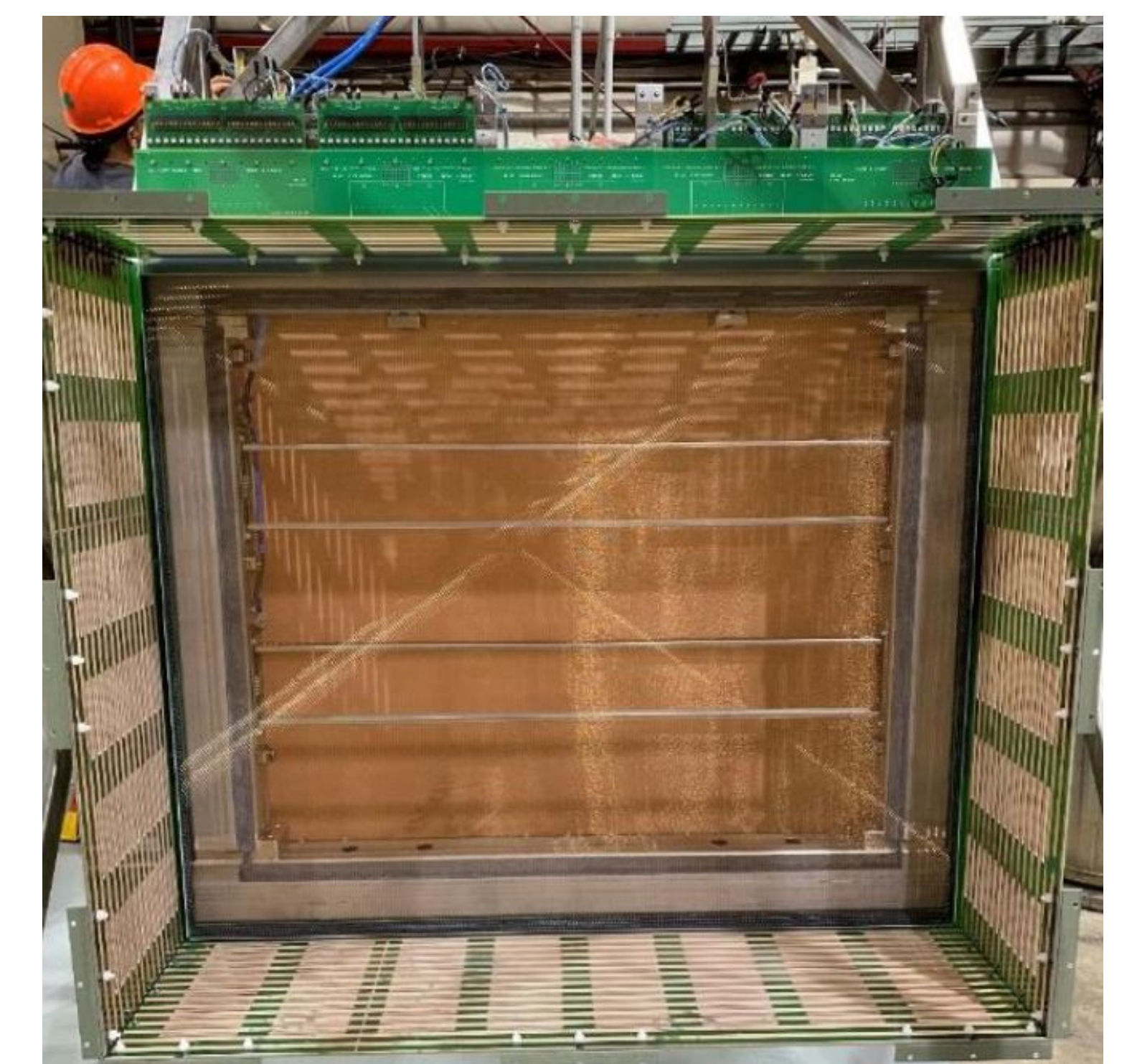
A picture of the inside of the ICEBERG detector, showing the surrounding field cage and photon detector slots. [3]
