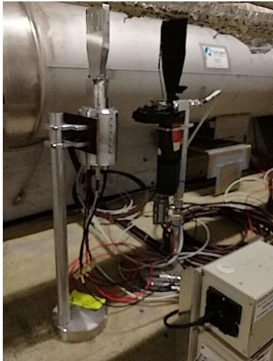
LHC BWS BEAM 1 PMT PART LIU type (right) OP type (left)
