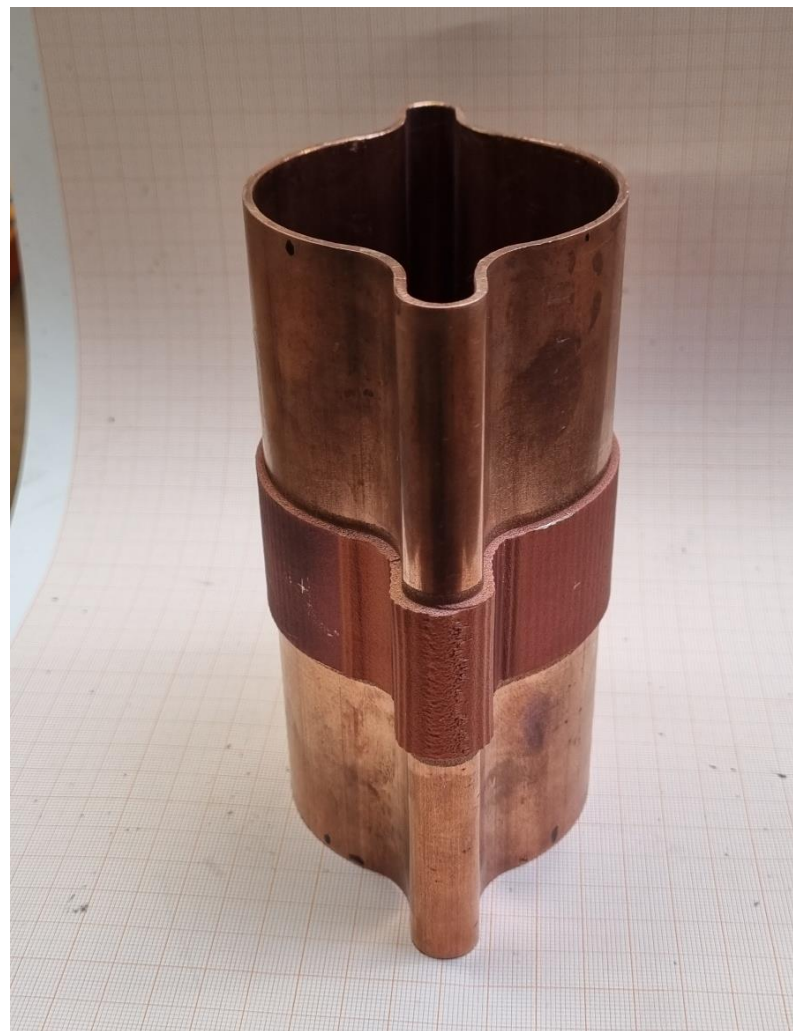
Chamber; 2mm layer sprayed all around
