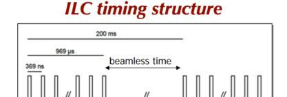
1 ms long bunch trains at 5 Hz2820 bunches per train308 ns spacing
