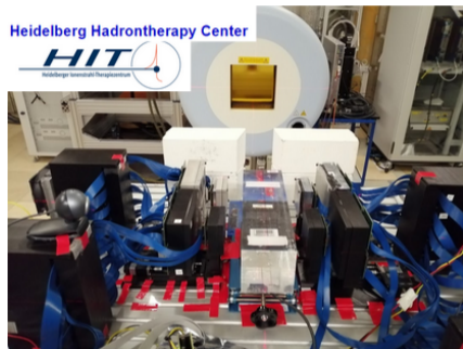
Figure 48: Four i-TED modules during a study under clinical conditions at the Heidelberg Hadrontherapy Center.
