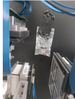
Figure 13: Experimental setup to study the background suppression applicability of different FoM. ^{22}\text{Na} source placed in front, side and back of i-TED-A module.
