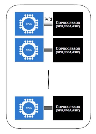
Also: workflows can only take advantage of acceleration if they run on a machine with a coprocessor – expensive at large scales!
