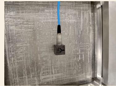
FTK accelerometers put on top of fiber plane and on frame
