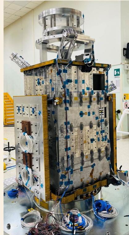
Vibrational tests of the whole spacecraft performed at Thales-Alenia in April 2024
