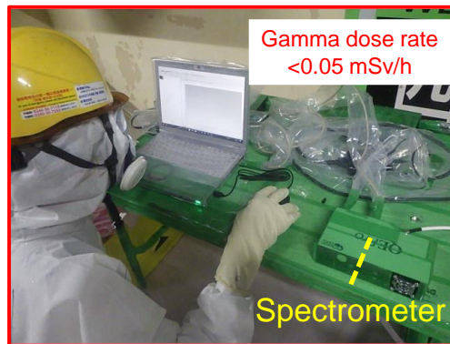
Fig. 1 Sensor installation condition inside the FDNPS Unit 3 reactor building.
