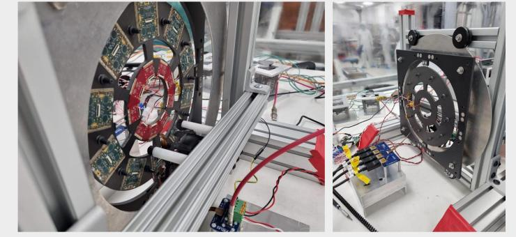
**Testing after Modules Loading** • Loaded modules RD53A are individually tested to assess any damages during loading • No performance degradation, no new disconnected bump-bonds found • Loading procedure is well-established and safe!
