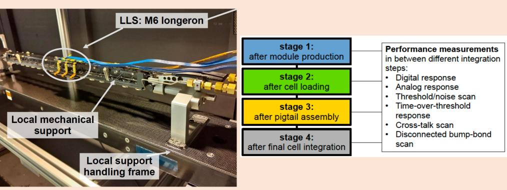
Demonstrator of loaded local support with RD53A modules and full services chain
