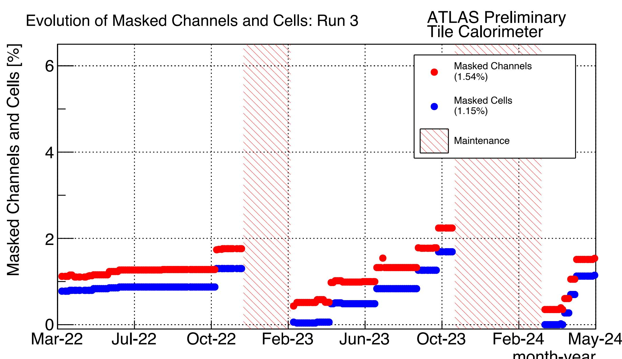
Continuous data quality activities and maintenance campaigns keep the fraction of non-functional readout channels below 2%.
