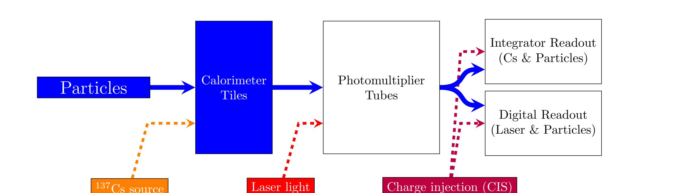
Charge-injection calibrates the readout electronics.
