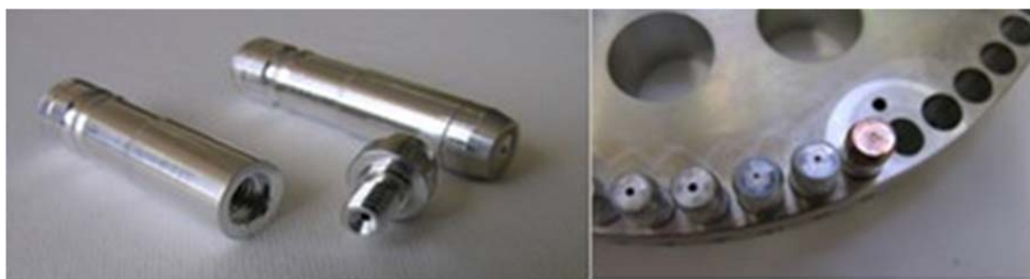
FIG. 10. Typical cathode systems used in the accelerator ion source for AMS studies, left is a cathode and right are cathodes in an ion source cathode wheel.
