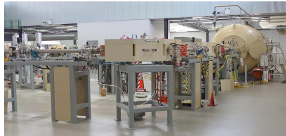
High energy beamlines for a 6MV Tandem Accelerator
