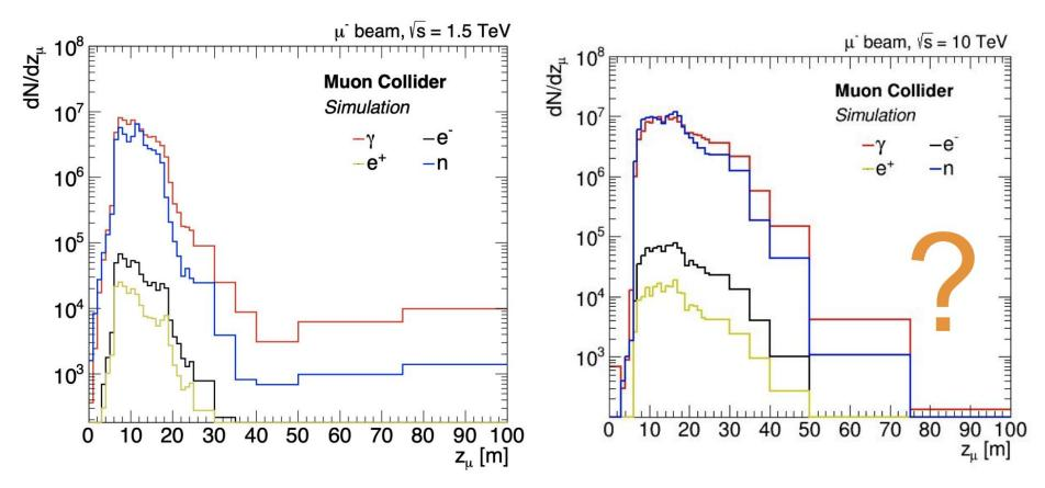
Lack of very-long tail comes from better modelling in FLUKA (now including synchrotron radiation)
