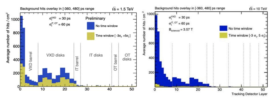
Increasing solenoid field to 5T has an effect of the order of 10% pre-timing
