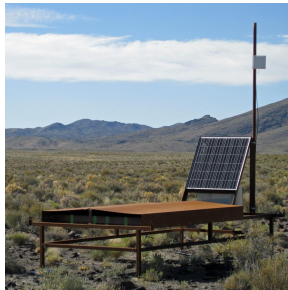
Telescope Array surface detector: a plastic scintillator
