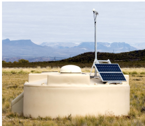
Auger surface detector: a water cherenkov tank
