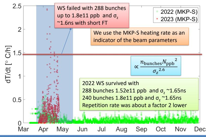
In 2023 the wire was exposed to unprecedented beam induced power. With the LIU target intensity the wire will be exposed to ~ factor 1.6 higher power loss
