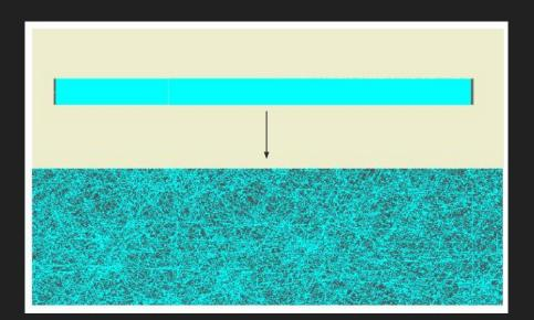
1 GeV muon in lead tungstate ~21,000 Cerenkov photons ~120,000 Scintillation photons  $\rightarrow$  Lots of computing power required!
