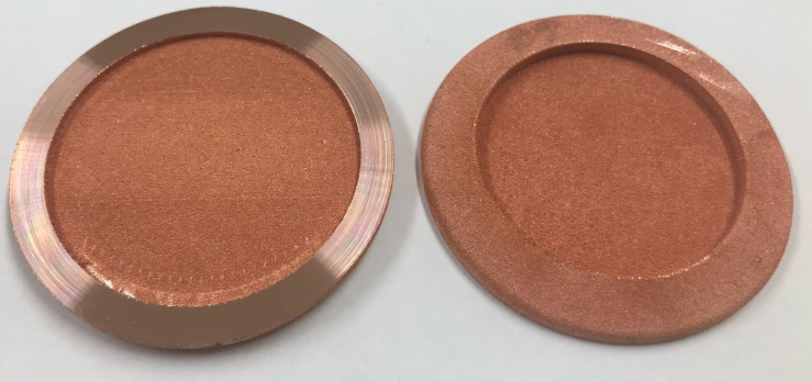
SR Absorber to be laser welded along outer profile
