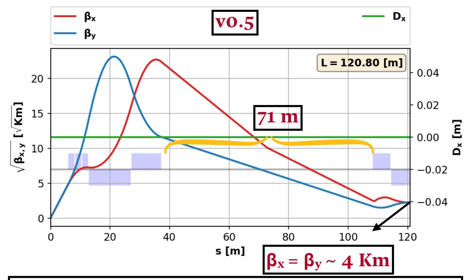
$B\rho = 16678.205 \ [Tm]$   $Aperture = 2(5\sigma + 0.02) \ [m]$   $\sigma_{j} = \sqrt{\frac{\beta_{j}\varepsilon_{nj}}{\beta_{r}\gamma_{r}}} + (D_{j}\delta_{p})^{2} \ [m] \ with \ j = x, y$   $\sigma = max(\sigma_{x}, \sigma_{y}) \ [m]$
